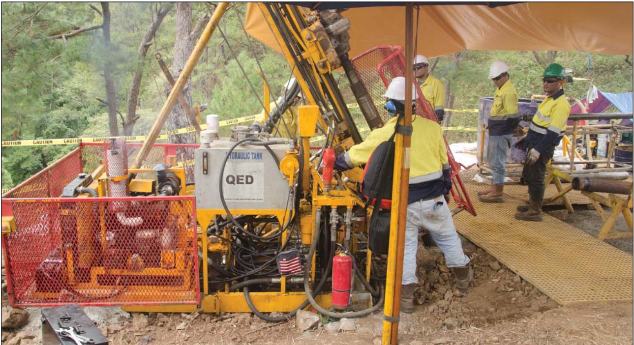
Figure 50: Well maintained MP500 diamond drill rig with a vertical depth capacity of 150 metres PQ, 300 metres HQ and 500 metres NQ
