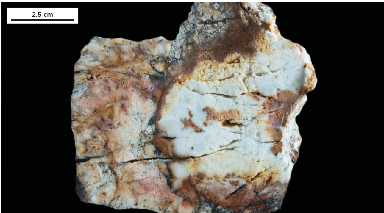
Figure 21: Fracture and edge oxidized white, cryptocrystalline to fine saccharoidal quartz. EAL sample ER01414 which assayed 0.68 g/t Au.
