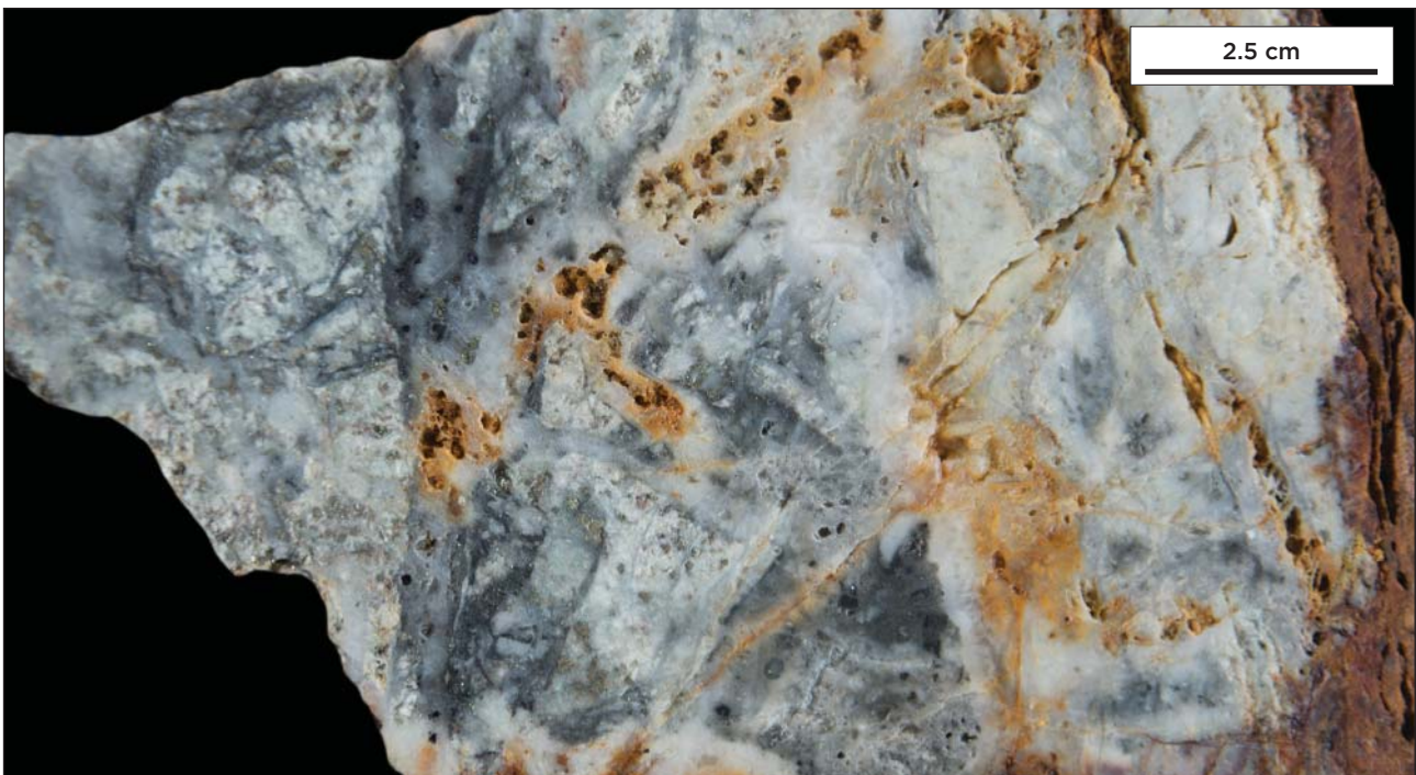
Figure 34: Strongly clay-silica minor pyrite altered diorite with pervasive stockwork of milk white to dark grey sulphidic quartz veinlets. Note patchy oxidation to limonite and vugs after sulphides. EAL sample ER01452 which assayed 34.68 g/t Au, 10.57 oz/t Ag and 0.22 % Pb.
