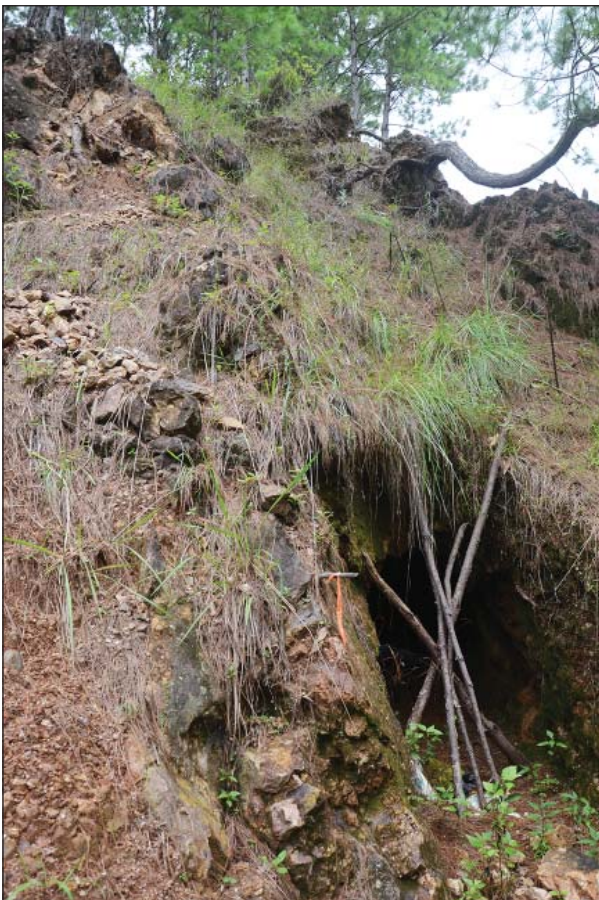
Figure 16: Abandoned artisanal adit at Danglay Ridge. Note that miners have targeted the edge of the quartz vein in the centre of the photograph.
