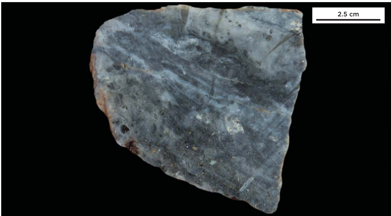
Figure 26: Grey to dark grey sulphidic quartz with small fragments of clay-silica altered wallrock. Note common blebby pyrite. EAL sample ER01454 which assayed 9.89 g/t Au, 2.59 oz/t Ag, 0.52 % Cu, 0.17% Pb and 0.18% Zn.
