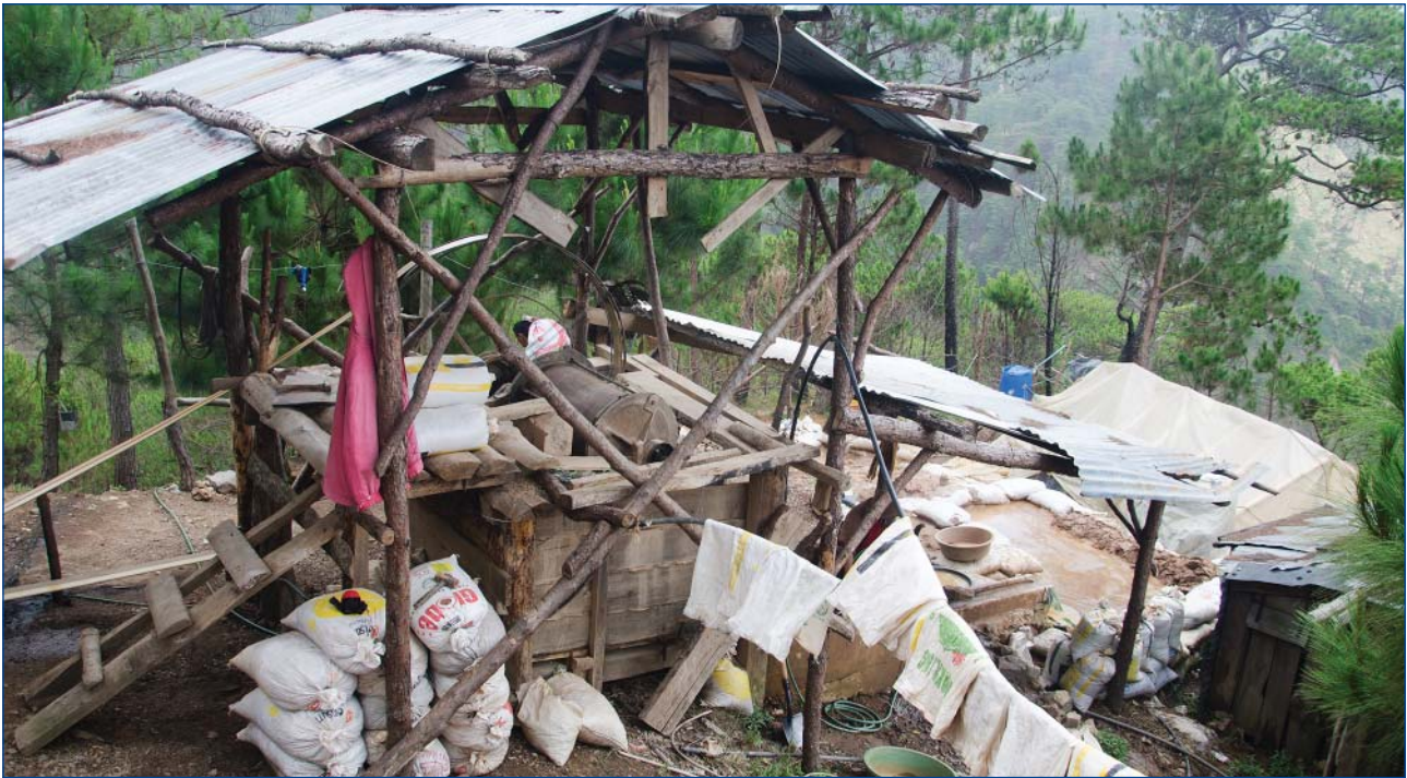
Figure 4: Typical artisanal plant comprising a very small locally-made ball mill, a gravity sluice box lined with 'miner's-matting' and a small settling pond. Artisanal plants throughout the Danglay prospect have minimal environmental impact and throughput is likely to be in the 10s of tonnes of oxide ore per annum.
