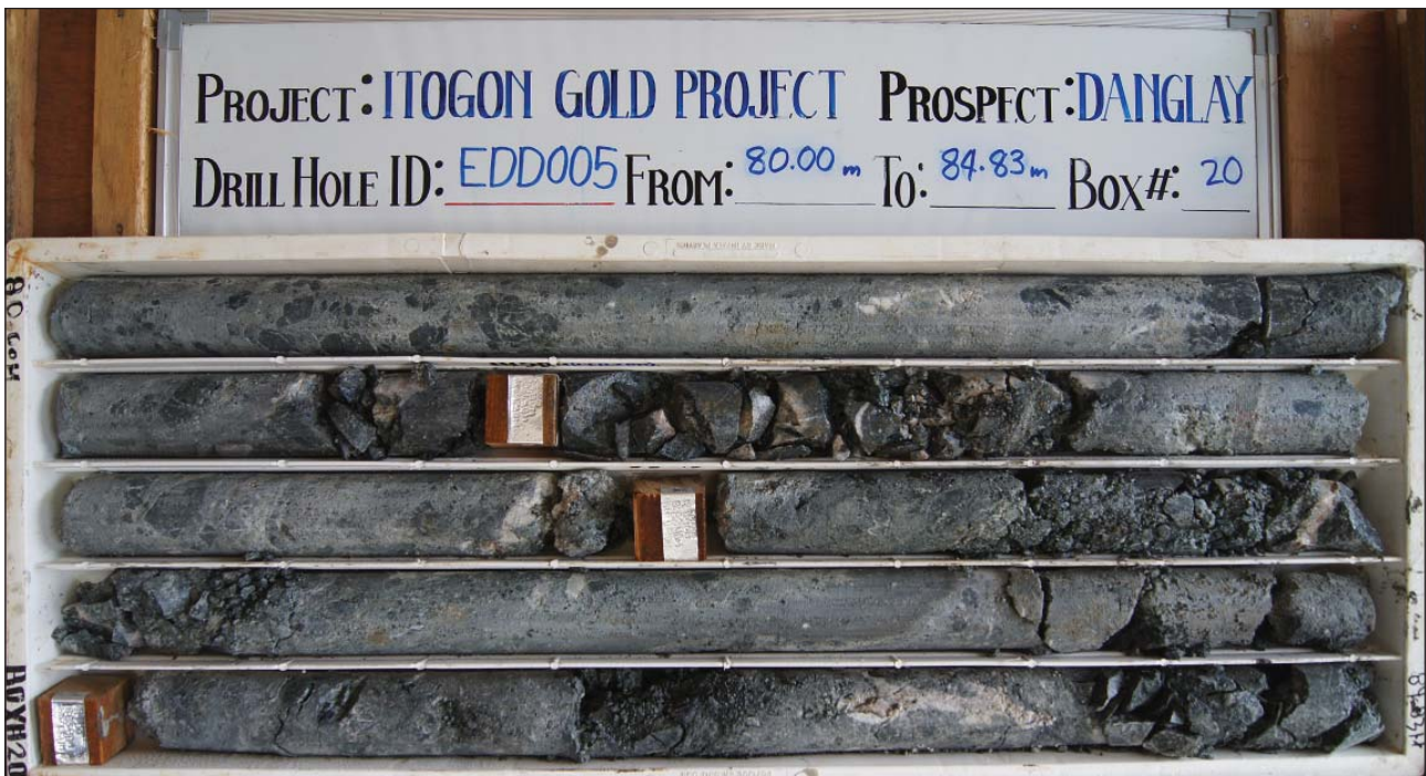
Figure 51: Example of the ECR diamond drill core stored in industry standard plastic trays. Note excellent core recovery even in broken ground.
