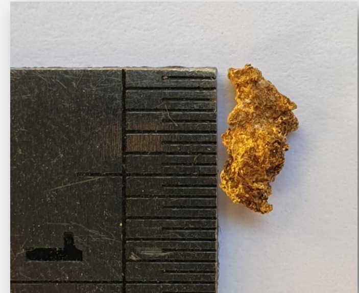
Above: nugget recovered in whole-of-bag gravity concentration trial.
