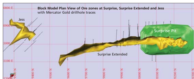
Surprise and Surprise Extended: zones coloured gold represents ore, blue represents waste and green represents the extent of historic open-pit mining
