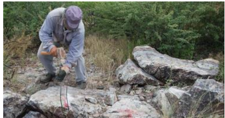
Channel Sampling the Main Vein: Maestro Aquerro 主矿脉上的刻槽取样
